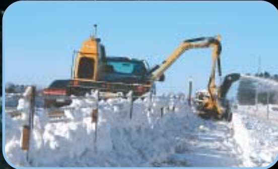
The Snow Panther's versatile hydraulic arm makes fast work of snow piles on either side of guard rail.
